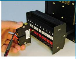
The DOC Drawout Case Test Plug provides an easy way to measure current and provide test access to GE style drawout case relays and meters. The DOC features normally-closed internal contacts. Upon insertion into the case, it brings the internal drawout case contacts out for easier access. Current Measurement Probes serve to redirect current circuits without disturbing them. Disconnect pins can be used to disable specific contacts and short-circuit currents.
