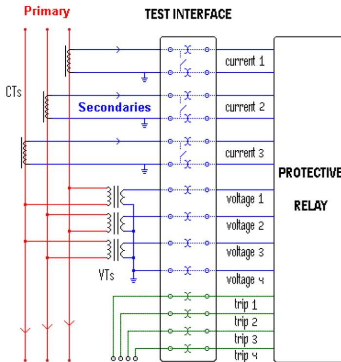
**Figure 1 – Conceptual wiring scheme for secondary circuits with integrated test interface**
