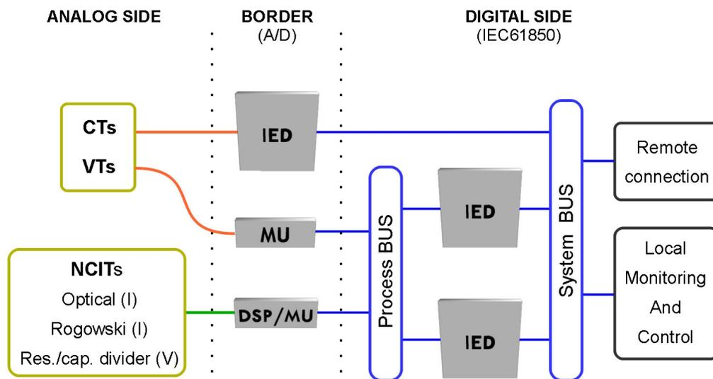
**Figure 2 – Analog to digital frontier in IEC61850 installations**
